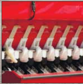
Seed is diverted into this tray for easy and accurate calibration
