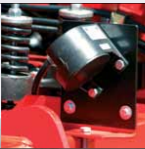
Radar for an accurate area count
