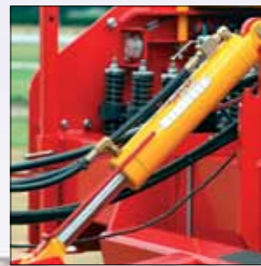
Hydraulic ram on the drawbar for easy adjustment
