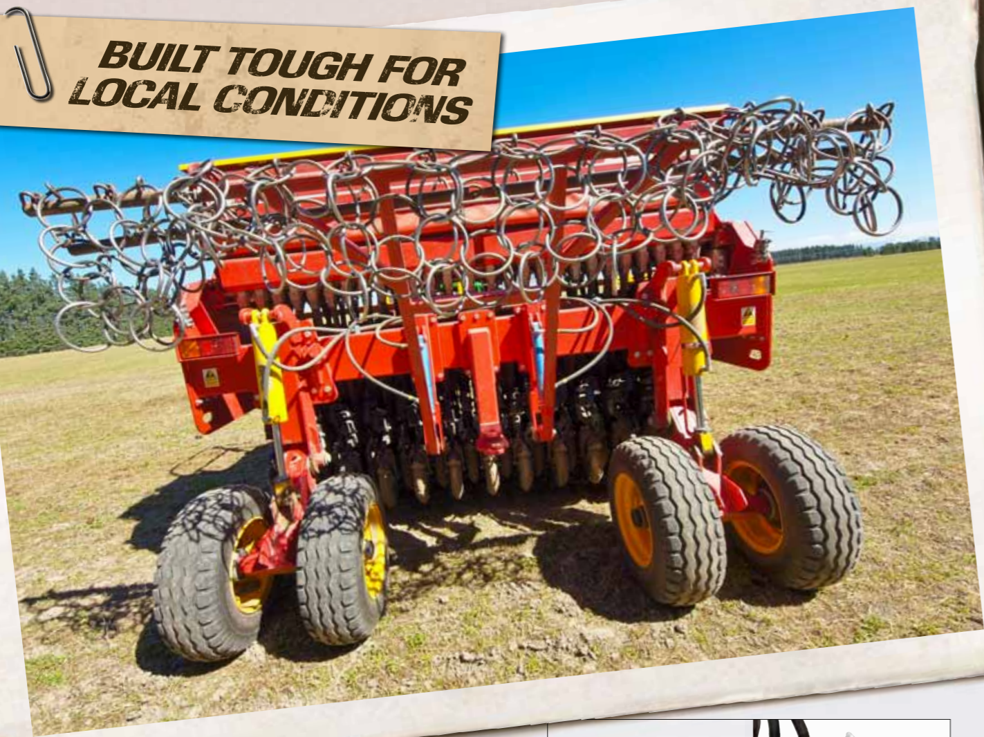
New parallelogram pivot bushes & new press wheel assemblies
