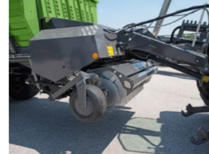
A hydraulic articulated drawbar gives the Tigo S a clearance of up to 70 cm.
