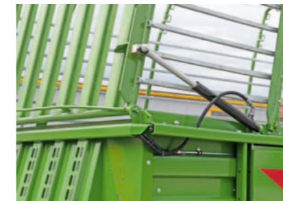
Another option is to have the collapsible dry feed assembly folded in and out hydraulically.
