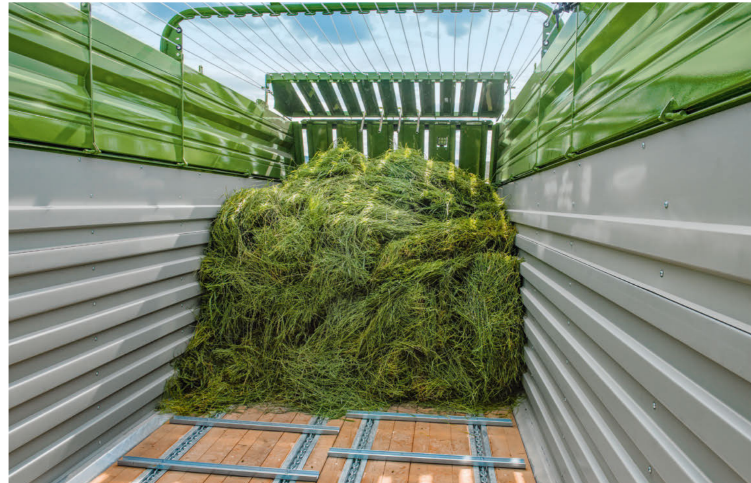
With the two-stage automatic loading system, light pressure is applied via a gauge bar, while moderate pressure is applied via the loading flap.
