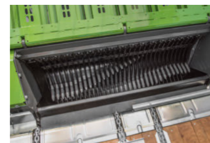
The rotor with a diameter of 800 mm and six spiral rows of teeth made of Hardox steel is equipped on both sides with large spherical roller bearings.
