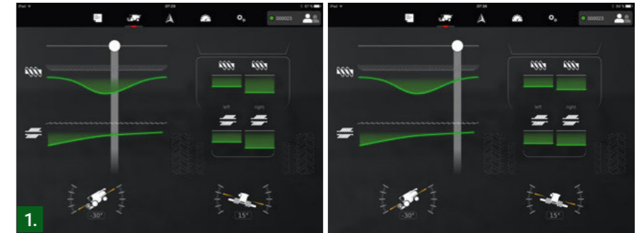
Detailed view of the Crop Load: the operator has a left/right view from the rear of the combine. Moving the slider along the length of the processor, it is possible to visualize the crop load in each area.
