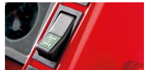
The rear differential lock prevents slipping and optimizes traction. The front traction disengagement is useful when travelling along roads and prevents damage from being done to delicate grounds.
