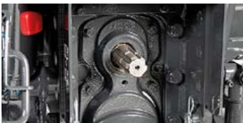
Two speed PTO: 540 rpm, 540 E (750 rpm) and synchronized with gear speeds. The PTO shaft of the ASAE 1 3/8 type is the same for all speeds.
