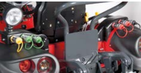
Hydraulic system with 4 double-acting manifolds, 1 single-acting, 1 continuous flow manifold + oil return tap.
