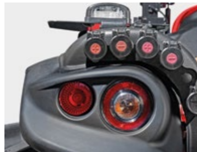
REAR QUICK COUPLERS Electro-proportional hydraulic system controlled by the "JPM" joystick, with dual operator safety system and integrated control unit with customizable configuration and settings - 12 rear couplers.
