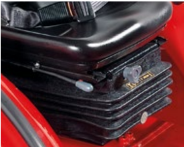
PNEUMATIC SEAT Latest generation with air springs.
