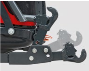
FRONT LIFT The front lift allows combined use of front and rear implements.
