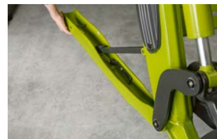
The support legs fold under the boom easily and do not obstruct the view of the front loader.
