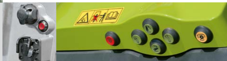
External controls for front and rear PTO
