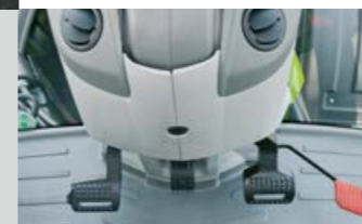
The steering column swings out of the way when the middle pedal is pressed.
