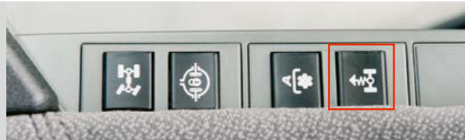
Switch to activate front axle suspension
