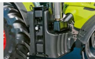
A ladder on the left-hand side provides safe access for cleaning and maintenance work.
