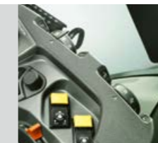
The working depth of the rear linkage is set using the dial on the armrest.
