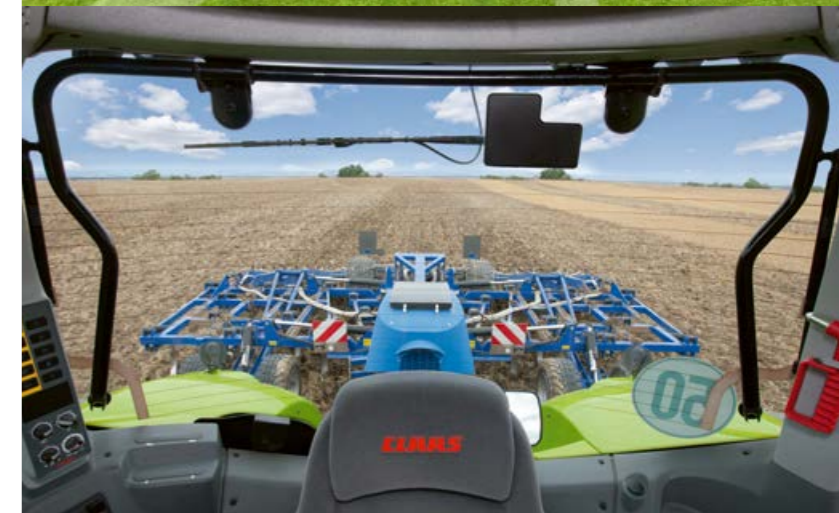
The convex rear window has a wide opening angle.
