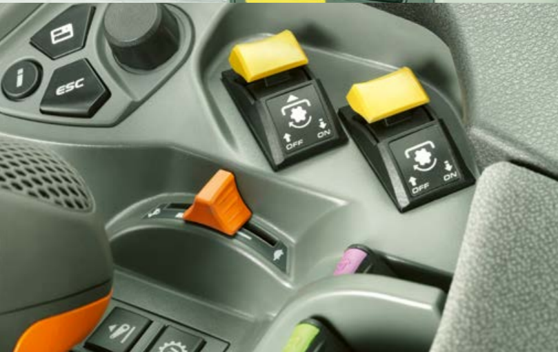
External controls for front and rear PTO
