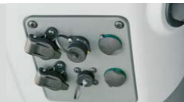
Connections to the power supply (25 A and cigarette lighter) and ISOBUS for additional terminals are located below the right-hand console.
