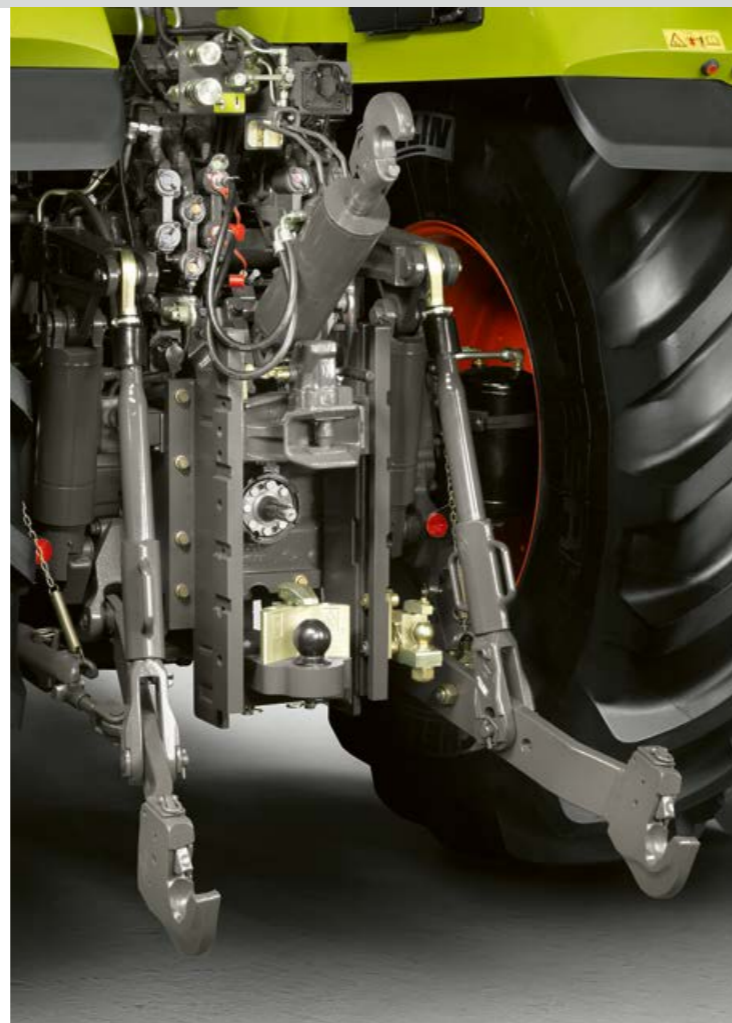
External controls for the rear linkage, PTO and one freely selectable spool valve
