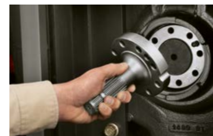
The PTO stub can be changed easily.
