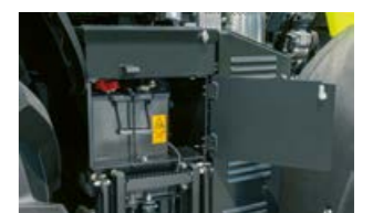
The battery is conveniently positioned above the right-hand access ladder.
