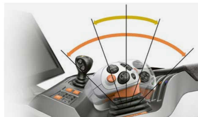
Shifting operation, powershift speeds + / - Shifting operation, range + / -
