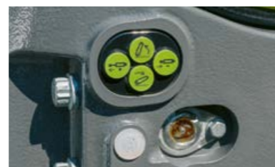
External controls for the front linkage and one spool valve in the CEBIS version.
