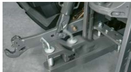
Several positions are available in the drawbar versions. The extended position improves manoeuvrability.
