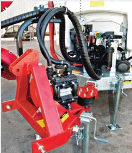
Pictured: Quantum Mist™ 2-row Sprayer with eight 500mm fan heads
