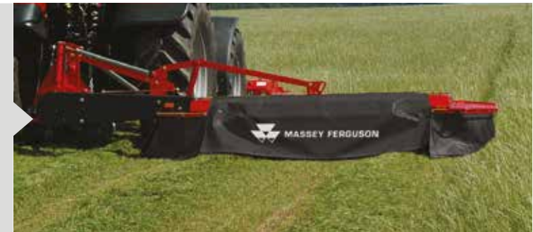
Rear-mounted, side attachment drum mower
