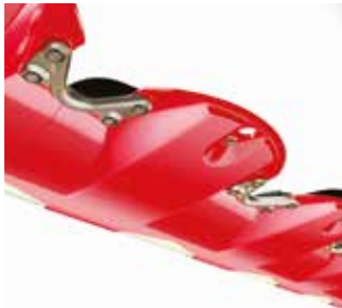
Streamline cutter bar (underside)
